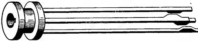
FIG. 3.—CAM FINGERS FOR TIGHTENING THE SEVERAL BANDS
